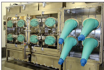
Figure 1: Mystic Pharmaceuticals' Versidoser™ intranasal unit dose Form-Fill-Seal production system.
